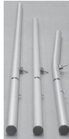
Above from left to right: Laser lower mast, Radial lower mast, and Laser 4.7 lower mast.
