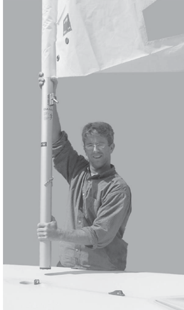
figure 30a: Stepping the Mast
