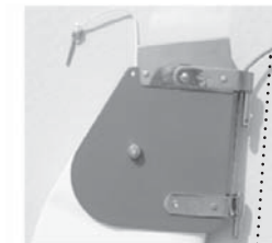
figure 76 | rudder downhaul line
